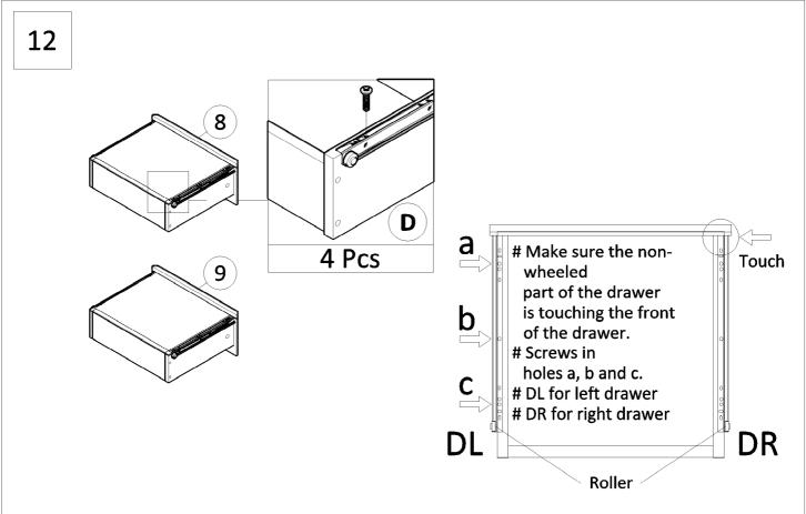
Failure to follow these directions could cause poor strength or stability. Insert screws loose to line up with slots then tighten up each screw.
