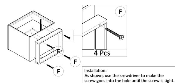
Failure to follow these directions could cause poor strength or stability. Insert screws loose to line up with slots then tighten up each screw.
