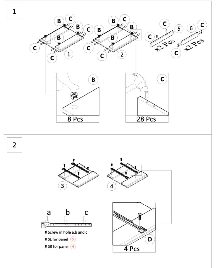
Failure to follow these directions could cause poor strength or stability. Insert screws loose to line up with slots then tighten up each screw.
